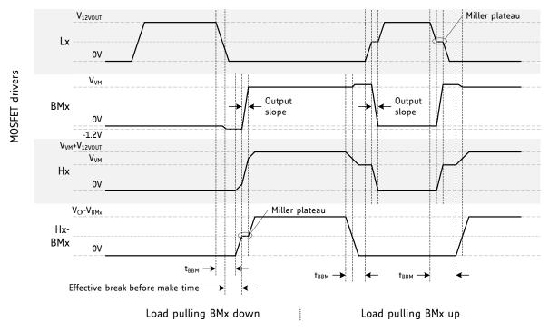
Figure 3.4 Slopes, Miller plateau and blank time
