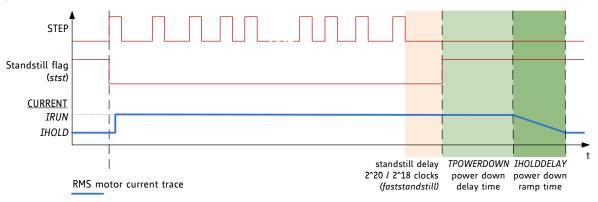
Figure 1.4 Automatic Motor Current Power Down
