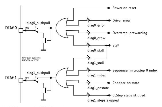
Figure 16.1 DIAG outputs in STEP/DIR mode
