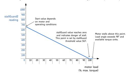
Figure 13.1 Function principle of StallGuard2
