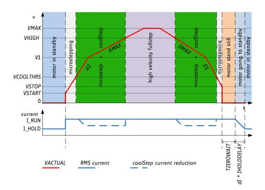
Figure 12.3 Ramp generator velocity dependent motor control
