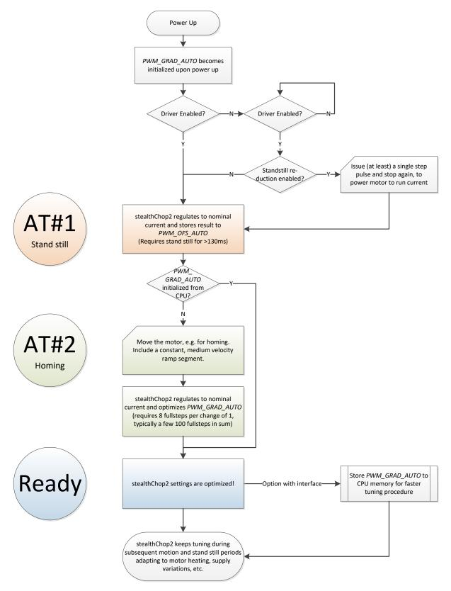
Figure 7.2 StealthChop2 automatic tuning procedure
