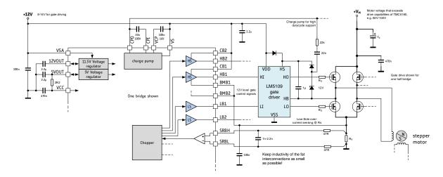
Figure 3.9 External Gate Driver Example
