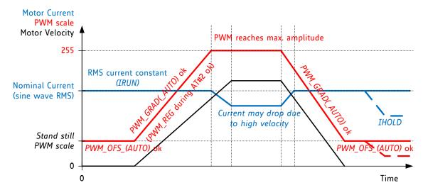
Figure 7.5 Successfully determined PWM\_GRAD(\_AUTO) and PWM\_OFS(\_AUTO)
