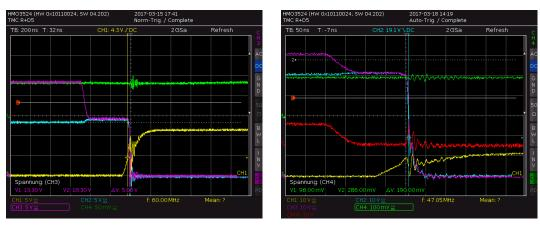
Figure 3.6 Ringing of output (blue) and Gate voltages (Yellow, Cyan) with untuned brige
