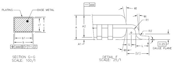
Figure 30.1 Dimensional drawings TQFP48-EP
