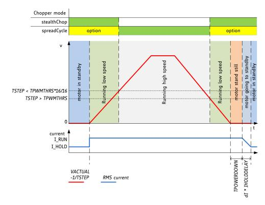
Figure 7.7 TPWMTHRS for optional switching to SpreadCycle
