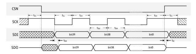
Figure 4.1 SPI timing
