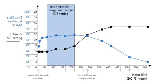
Figure 13.2 Example: optimum SGT setting and StallGuard2 reading with an example motor
