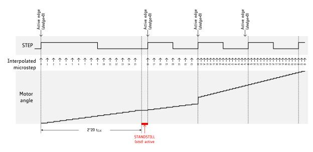
Figure 15.2 MicroPlyer microstep interpolation with rising STEP frequency (Example: 16 to 256)
