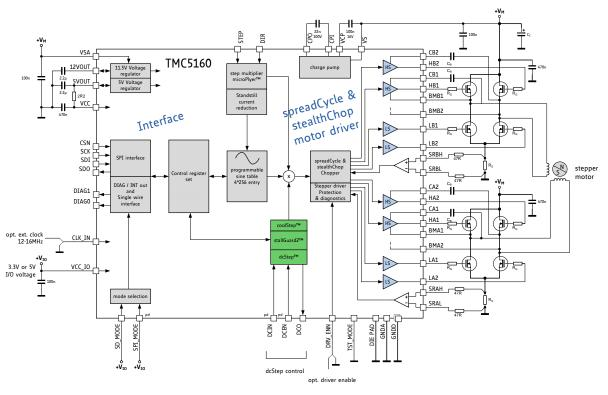
Figure 1.2 TMC5160 STEP/DIR application diagram
