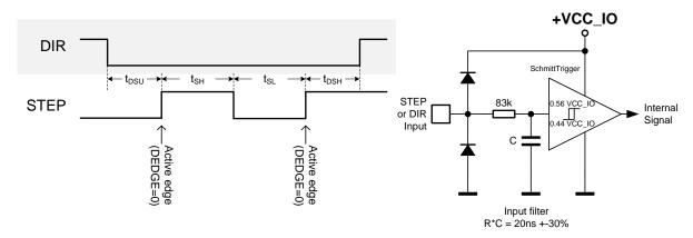
Figure 15.1 STEP and DIR timing, Input pin filter
