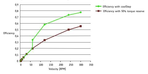
Figure 1.5 Energy efficiency with CoolStep (example)
