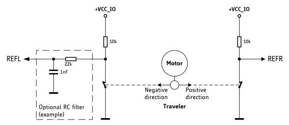
Figure 12.4 Using reference switches (example)
