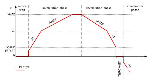
Figure 12.1 Ramp generator velocity trace showing consequent move in negative direction
