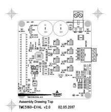
The TMC5160-EVAL is part of TRINAMICs universal evaluation board system which provides a convenient handling of the hardware as well as a user-friendly software tool for evaluation. TMC5160 evaluation board system consists οf three parts: LANDUNGSBRÜCKE (base board), ESELSBRÜCKE (connector board including several test points), and TMC5160-EVAL.
