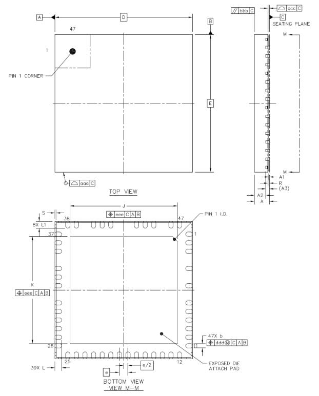
Figure 30.2 Dimensional drawings wettable QFN
