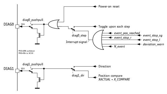
Figure 16.2 DIAG outputs with SD\_MODE=0
