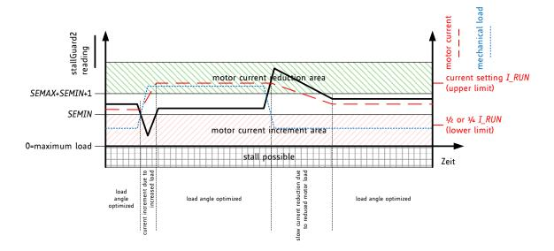
Figure 14.1 CoolStep adapts motor current to the load
