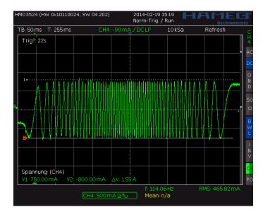
Figure 7.3 Scope shot: good setting for PWM\_REG
