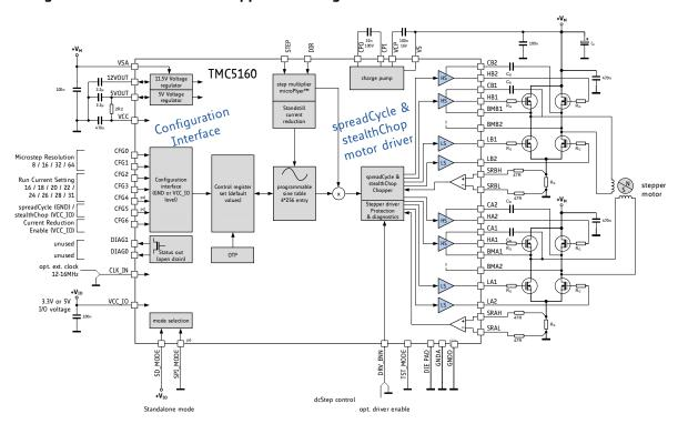
Figure 1.3 TMC5160 standalone driver application diagram
