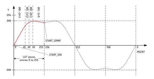
Figure 18.1 LUT programming example
