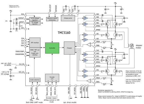
Figure 3.1 Standard application circuit
