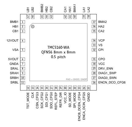
Figure 2.2 TMC5160-WA package and pinning QFN-WA (8x8mm²)
