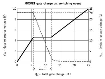
Figure 3.3 Miller charge determines switching slope
