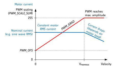
Figure 7.6 Velocity based PWM scaling (pwm\_autoscale=0)
