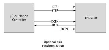
Figure 17.4 Full signal interconnection for DcStep
