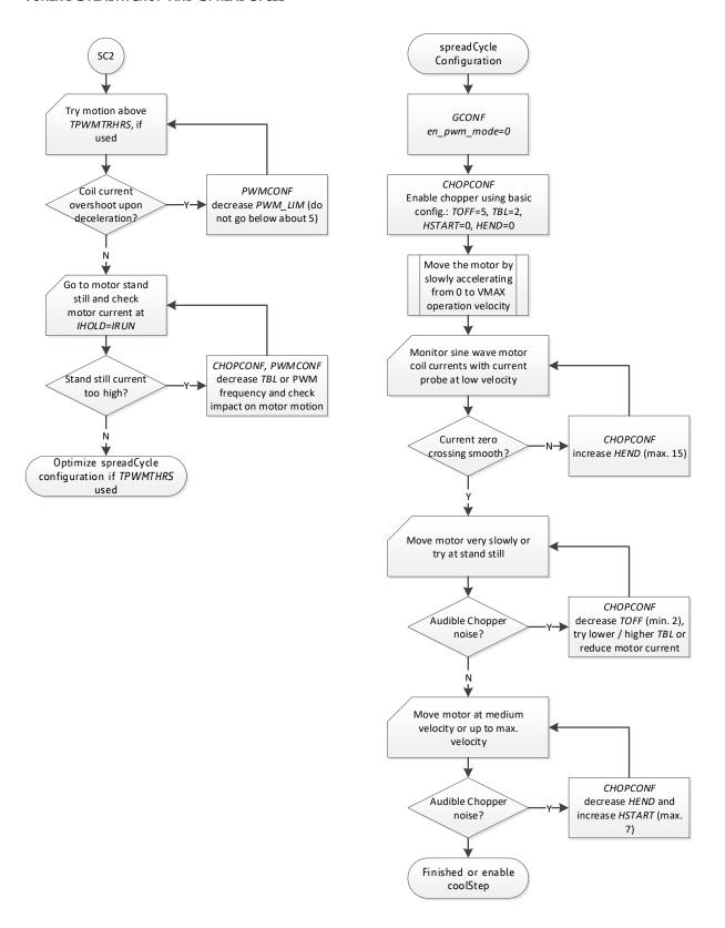
Figure 22.2 Tuning StealthChop and SpreadCycle
