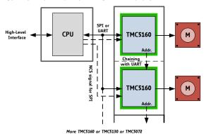
An application with 2 stepper motors is shown. Additionally, the ABN Encoder interface and two reference switches can be used for each motor. A single CPU controls the whole system, as there are no real time tasks required to move a motor. The CPU-board and the controller / driver boards are highly economical and space saving.
