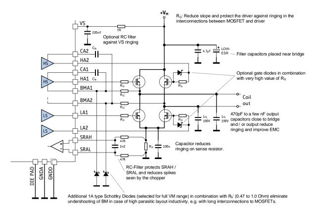
Decide use and value of the additional components based on measurements of the actual circuit using the final layout!
