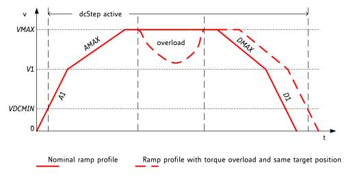
Figure 17.2 Velocity profile with impact by overload situation
