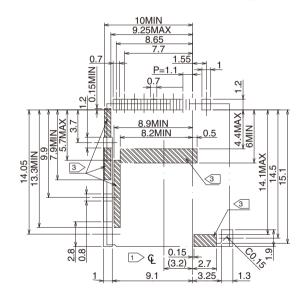
Note 1  $\bigcirc$  indicates the center line of the microSD card slot.
