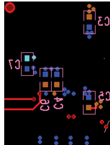
Figure 90. Bottom Layer Decoupling
