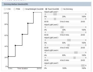
Allow users to separate 24hrs into 5 sections and corresponding output current.
