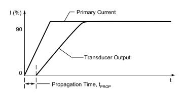
**Propagation Delay (t<sub>PROP</sub>)**
