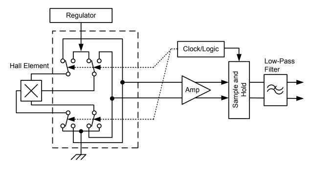
**Concept of Chopper Stabilization Technique**
