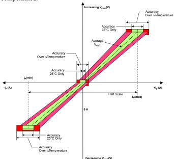
Output Voltage versus Sampled Current Total Output Error at 0 A and at Half-Scale Current
