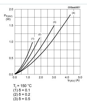
Fig. 7. Average forward power dissipation as a function of average forward current; typical values
