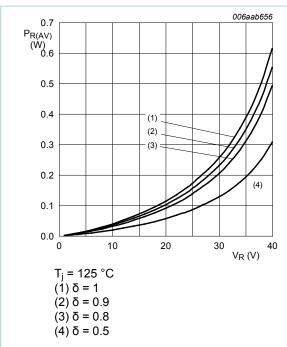
Fig. 8. Average reverse power dissipation as a function of reverse voltage; typical values
