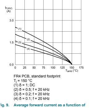
Fig. 9. ambient temperature; typical values
