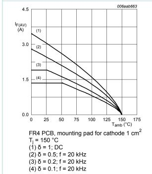
Fig. 10. Average forward current as a function of ambient temperature; typical values
