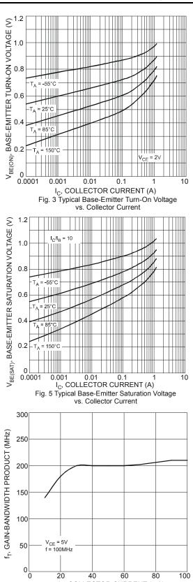
I<sub>C</sub>, COLLECTOR CURRENT (mA) Fig. 7 Typical Gain-Bandwidth Product vs. Collector Current
