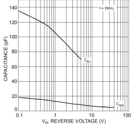
Fig. 6 Typical Capacitance Characteristics
