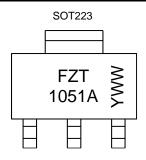
FZT 1051A = Product Type Marking Code YWW = Date Code Marking Y or  $\overline{Y}$  = Last Digit of Year (ex: 9 = 2019) WW or  $\overline{W}W$  = Week Code (01 to 53)
