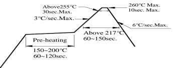
3.2 Reflow soldering should not be done more than two times.
