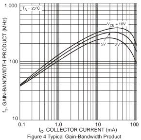
Figure 4 Typical Gain-Bandwidth Product vs. Collector Current
