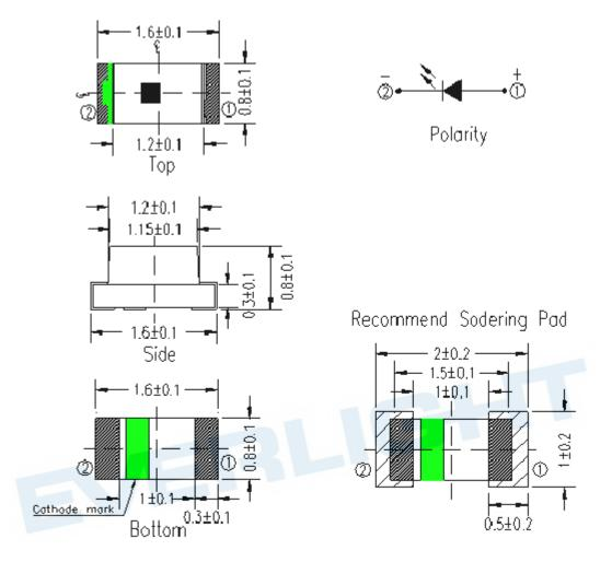
Suggested pad dimension is just for reference only. Please modify the pad dimension based on individual need. Note: Tolerances unless mentioned ±0.1mm. Unit = mm
