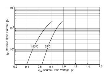
Figure 4. Output Characteristics
