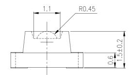
For reflow soldering (propose)
