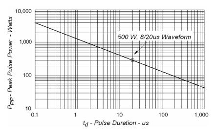
Fig1. Peak Pulse Power VS Pulse Time
