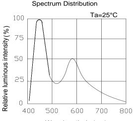
$Wave length \ \lambda p(nm) \\ Relative Luminous Intensity vs.$
