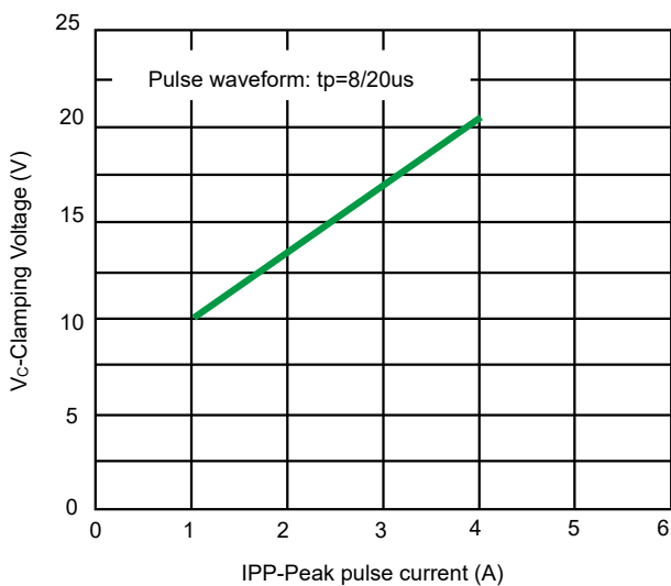
Fig 5. Clamping voltage vs. Peak pulse current
