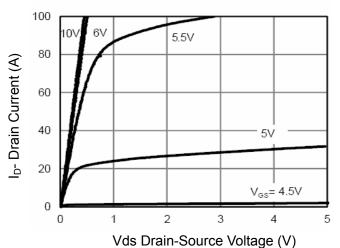
**Figure 1 Output Characteristics**
