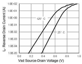
Figure 6 Source- Drain Diode Forward
