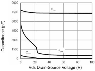
Figure 7 Capacitance vs Vds
