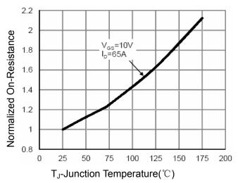
**Figure 4 Rdson-Junction Temperature**
