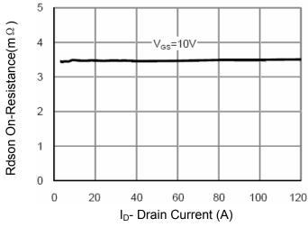
Figure 3 Rdson- Drain Current
