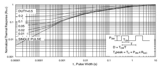
Figu11. Normalized Maximum Transient Thermal Impedance
