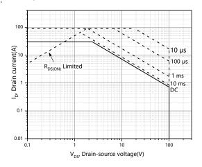
Figure 9, Drain current
