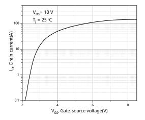
Figure 1, Typ. output characteristics
