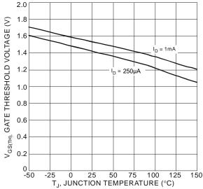
Figure 6. Gate Threshold Variation vs. Junction Temperature
