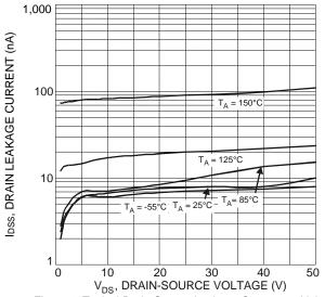
Figure 8. Typical Drain-Source Leakage Current vs. Voltage
