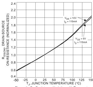
Figure 4. On-Resistance Variation with Temperature
