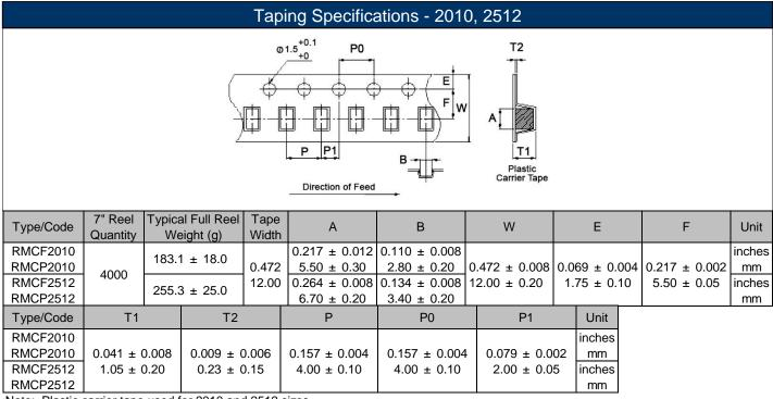
Note: Plastic carrier tape used for 2010 and 2512 sizes.
