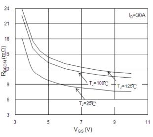
Fig.2 On-Resistance vs. Gate-Source
