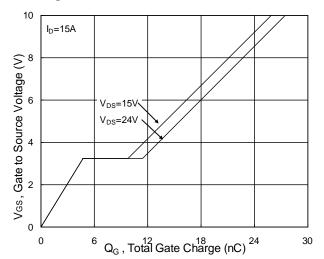
**Fig.4 Gate-Charge Characteristics**
