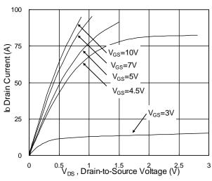
**Fig.1 Typical Output Characteristics**
