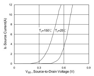
Fig.3 Forward Characteristics of reverse
