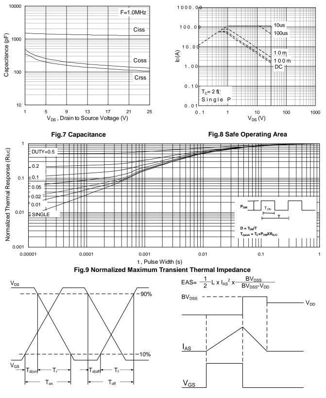
Fig.10 Switching Time Waveform
