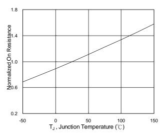
Fig.6 Normalized R<sub>DSON</sub> vs. T<sub>J</sub>
