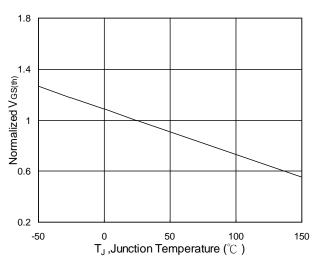
Fig.5 Normalized  $V_{GS(th)}$  vs.  $T_J$
